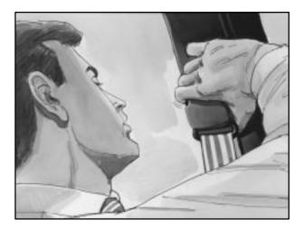
To move it down, squeeze the release button and move the height adjuster to the desired position. You can move the adjuster up just by pushing up on the shoulder belt guide. After you move the adjuster to where you want it, try to move it down without squeezing the release button to make sure it has locked into position.
